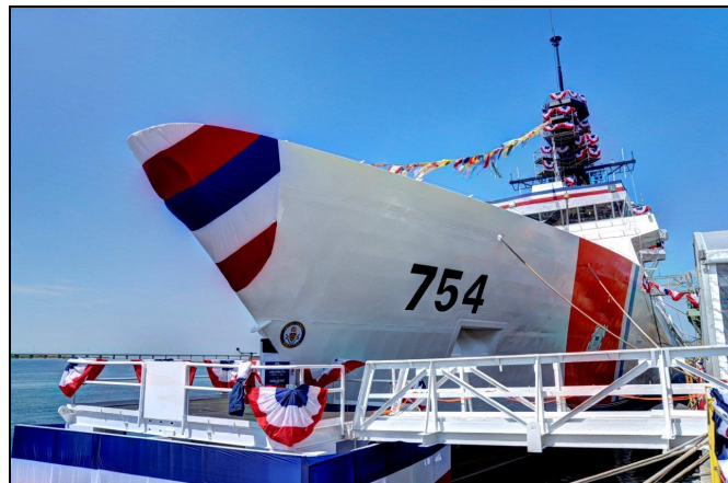
The National Security Cutter is 418 feet long with a maximum beam (width) of 54 feet. It has a range of 12,000 nautical miles, a crew of 110 personnel, and can carry two helicopters and three small boats. The ship has a propulsion plant consisting of two diesel engines and a gas turbine producing a total of 50,000 shaft horsepower.
